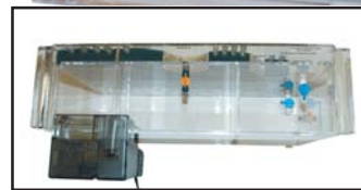
Top view of reservoir tank with pump in position.
